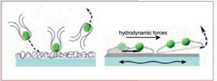
Figure 1. Illustrative scheme of antifouling and fouling release processes.
